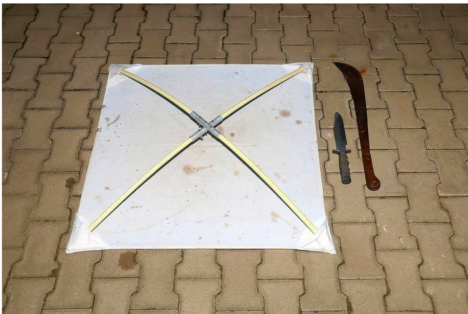
Fig. 2. The assembled beating sheet, ready for use. The plastic pipes are under tension with the cross about 20 cm above the sheet
