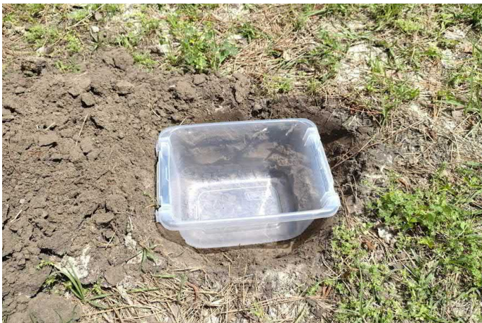
Fig. 4. The container is set in the ground at the same level as the surface of the surrounding soil.
