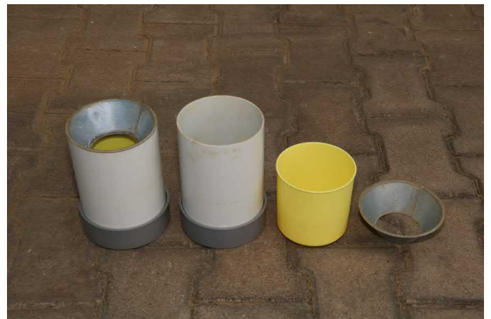
Fig. 2. The latter much-improved design, with white pipe and metal funnel. This is the version I still use.
